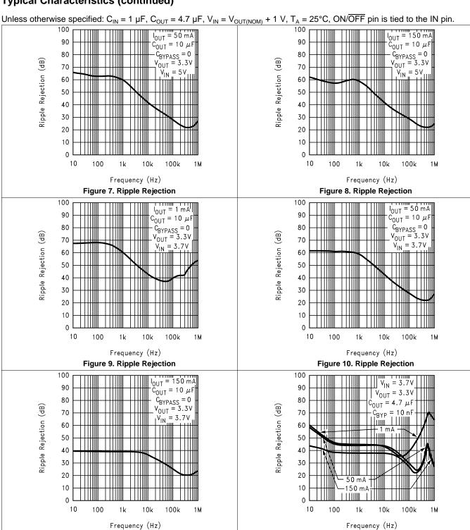
Figure 11. Ripple Rejection
