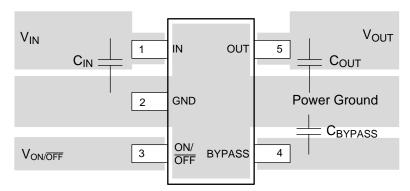
Figure 42. LP2992 SOT-23 Package Typical Layout
