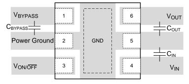
Figure 43. LP2992 WSON Package Typical Layout
